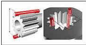
Example of two measuring pins on both external and internal gears with an even number of teeth
